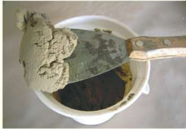
Mix 4 volumes of Brush Coat and 1 volume of water to a paste
